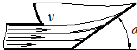
Fig. 2. Trajectory behavior of layer moving in the canal in the impingement on oblique plane obstacle
